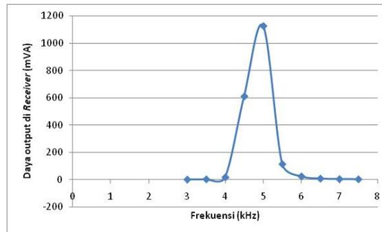
Fig.3.Frequency response of power at the receiver.
