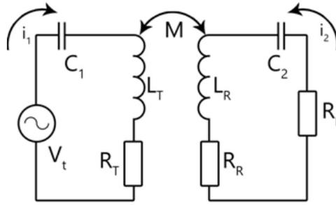
Fig.1. Equivalent circuit of coupled magnetic resonance.
