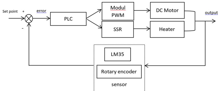
Fig. 1. Block diagram of hardware design
