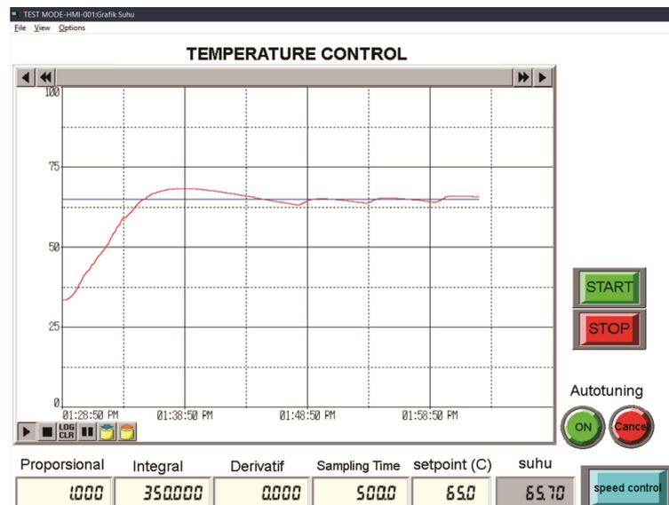
**Fig. 7.** Temperature control testing result
