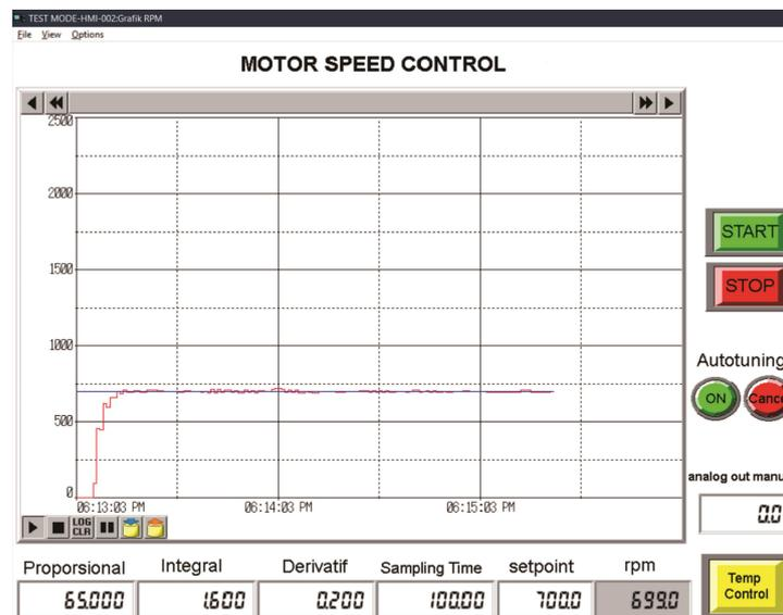
Fig. 6. Motor speed control testing result
