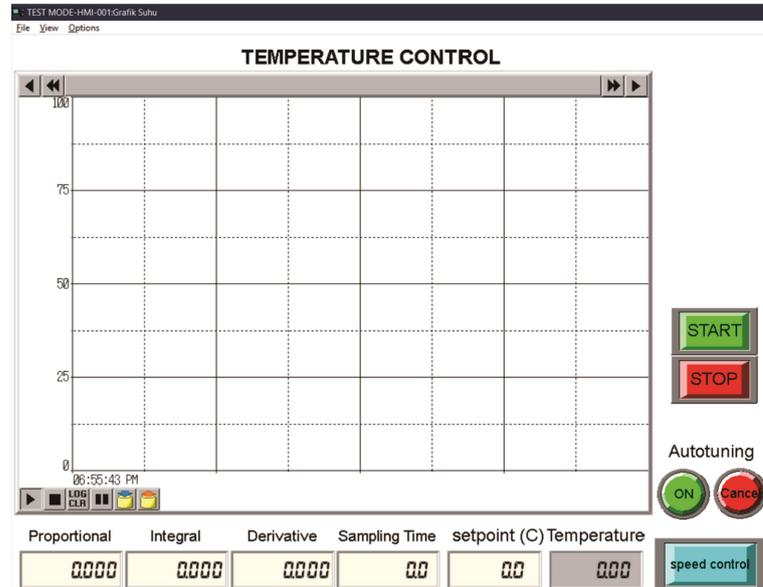
Fig. 4. Temperature control interface page
