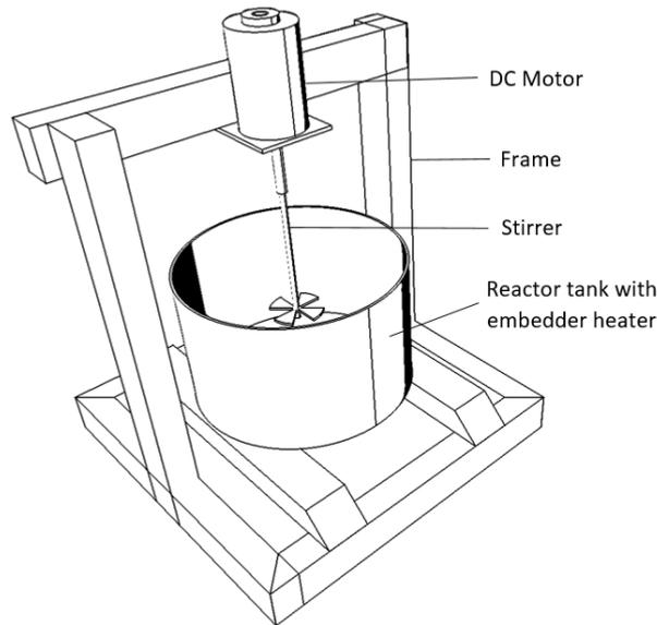
Fig. 2. Biodiesel reactor prototype design
