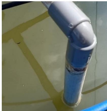
Fig. 5. Turbidity sensor testing
