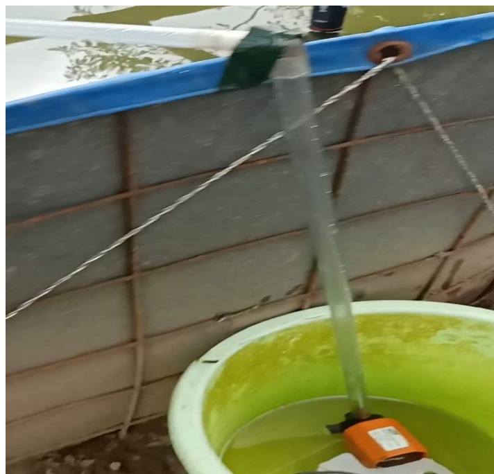
Fig. 9. pH sensor testing
