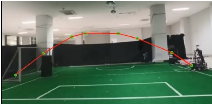
Fig. 7. Lever kick distance of 14 cm
