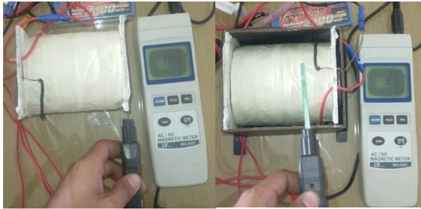
Fig. 9. Value of the magnetic field on a solenoid without a cover
