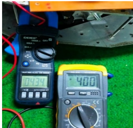
Fig. 6. Voltage and current in the solenoid kick mechanism
